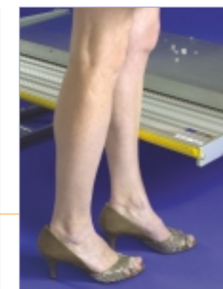
Sensitive edge protects vulnerable passengers.
