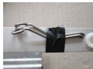
Water proof connectors Nylon bearing (right) Anti-rattle springs (Below)
