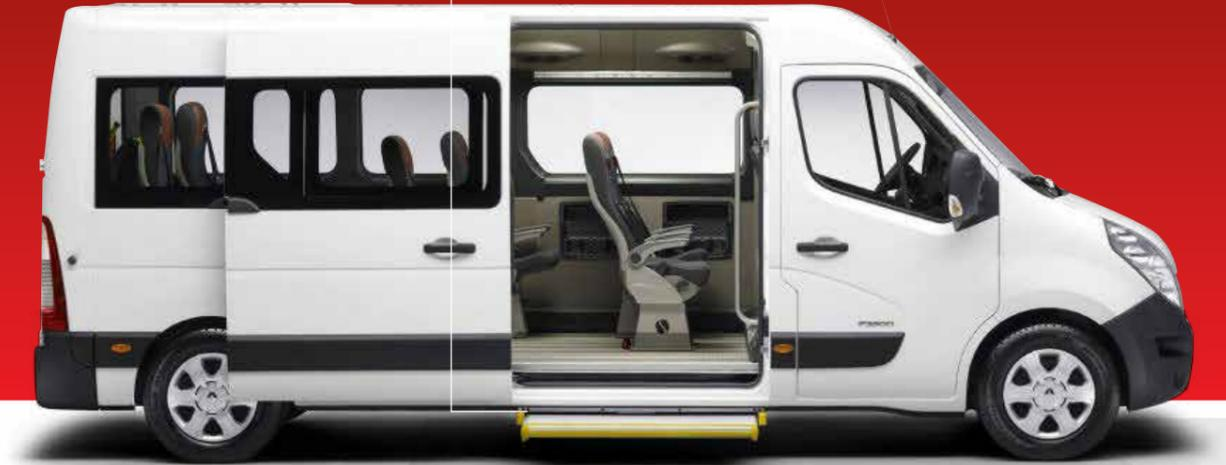
**Illuminated top edge** - ribbon switch lights up step when deployed and vehicle lights are on
